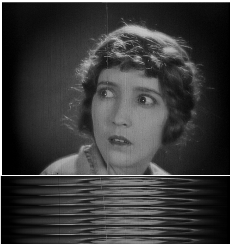
Fig. 3. Image from the “lost world” movie and projected image P(x, y) for 7 consecutive frames. The projection height H is 16. The scratches (dark one on the left side, bright one and dark one in the middle) are still visible.
