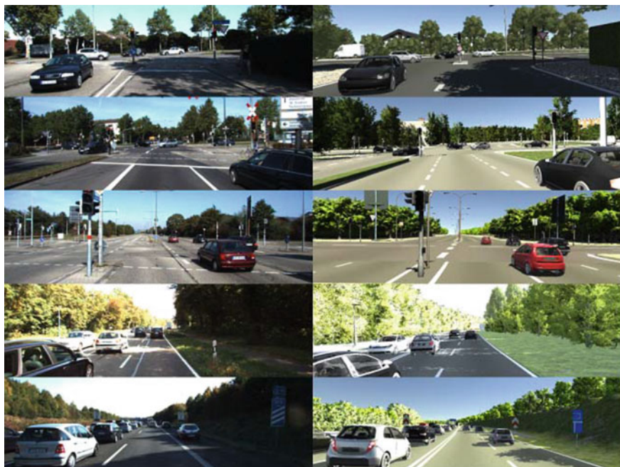
Fig. 19 Frames from 5 real KITTI videos (first column) and the corresponding virtual clones (second column) ( source Gaidon et al., 2016)
