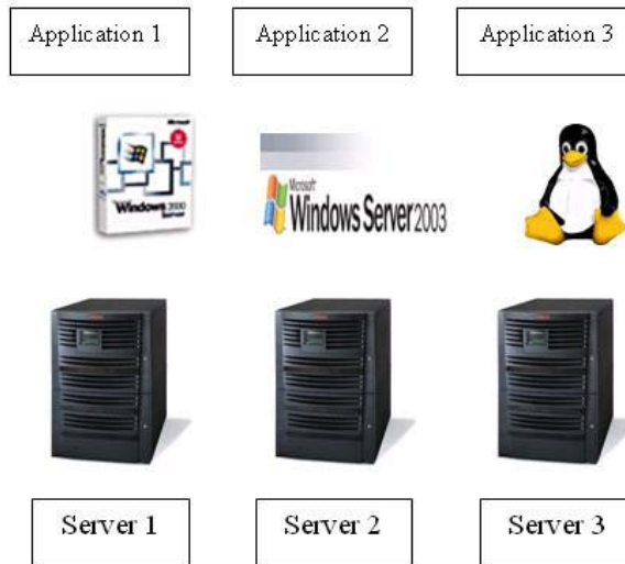
Figure 7.1. A Non-virtualized environment: three physical servers, three different operating systems, and three applications running on separate machines
