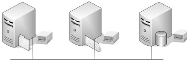
Figure 10.4. Backup on LAN via backup server (only one tape)
