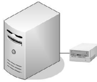
Figure 10.3. Local backups on LAN (each desktop or server has its own tape)
