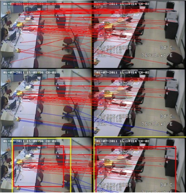
Fig. 5. SIFT-based Keypoint Detection and Matching between Wide Angle Camera (Left) and PTZ Camera (Right)
