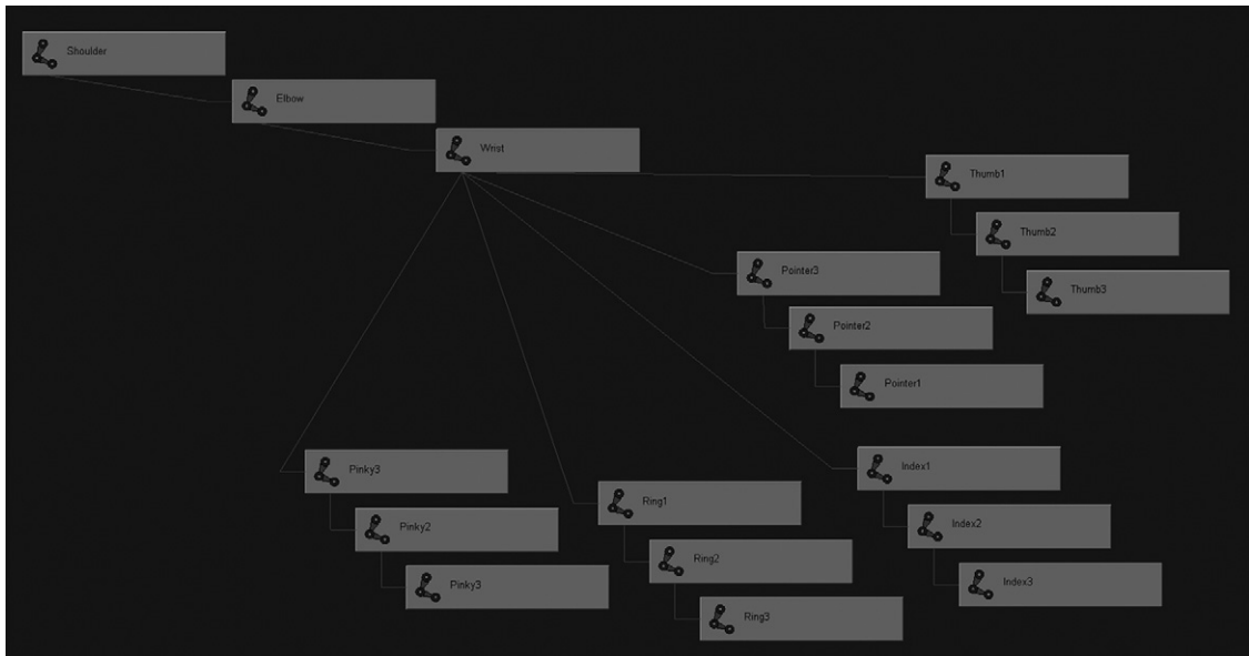
Figure 17.4 Graph showing the hierarchy of a joint system from the shoulder down to all of the fingers.
