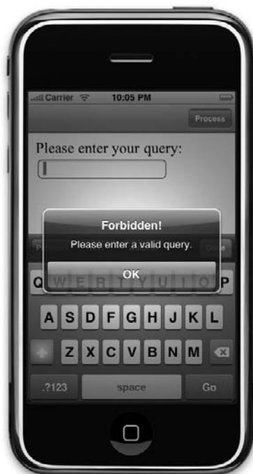
Figure 8.17 A screenshot of the application that demonstrates JavaScript execution from within Objective-C code. The screenshot shows an alert view when a forbidden query is used.
