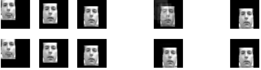
Fig. 3. Least squares reconstructions of a target image (far right) from three nearby images (left). The intermediate (fourth) image shows the best least squares reconstruction of the rightmost image from the three leftmost images. First row: standard reconstruction. Second row: reconstruction after local transformations.
