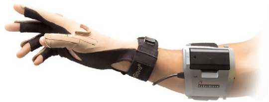
Figure 1.17 The Cyberglove II. Photo courtesy of Cyberglove Systems LLC.
