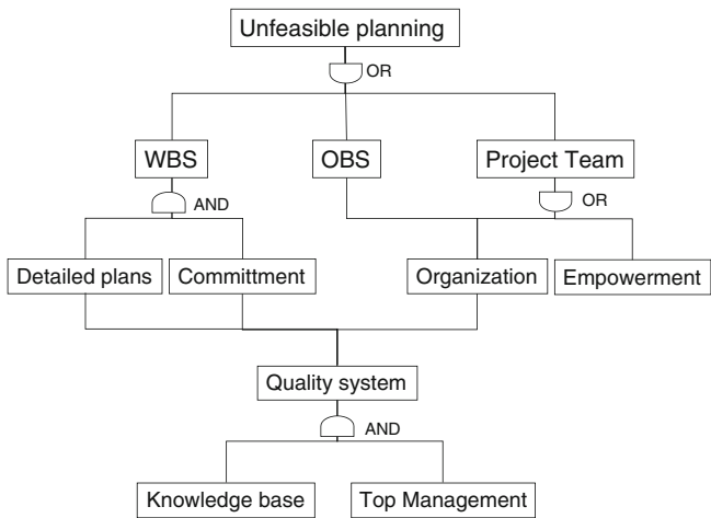
Fig. 14.1 Example of fault tree analysis
