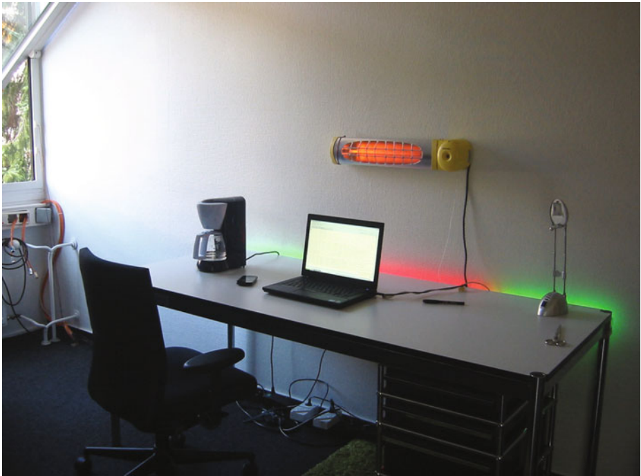
Fig. 1. Center of the desk is augmented with red light because the heater is switched on while the window is open. Left and right part are augmented with green light since the coffee machine and desk lamp are switched off (best viewed in color).
