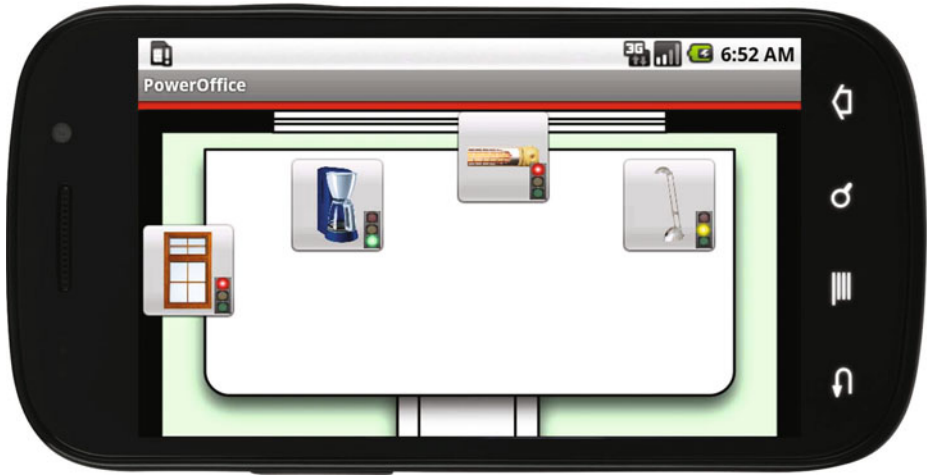
Fig. 2. Overview of the office environment. The traffic lights indicate which object has energy-saving potential (best viewed in color).
