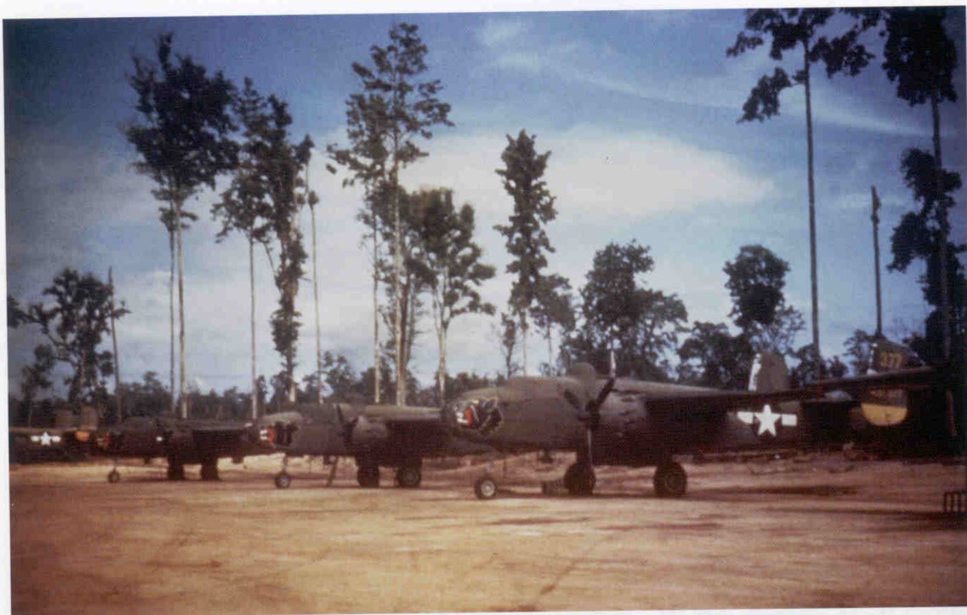
Above: These B-25Js have the solid noses with the eight .50-caliber machine guns installed. The black panther nose art indicates that they are assigned to the 501st Bomb Squadron of the 345th Bomb Group.
