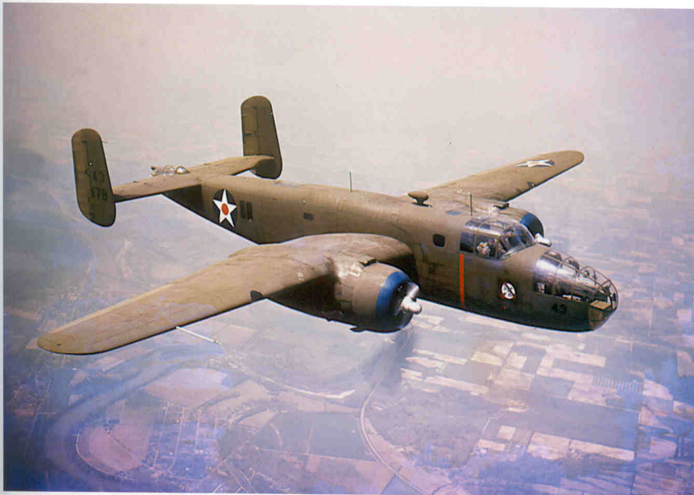
Above: The Thunderbird insignia of the 17th Bombardment Group's 34th Bombardment Squadron is displayed on the nose of this B-25A. The 17B on the vertical tail indicates the 17th BG, while the 43 on the vertical tail and nose is the aircraft's number within the unit. Note the early style national insignia with the red disc at its center. (via Piet)
