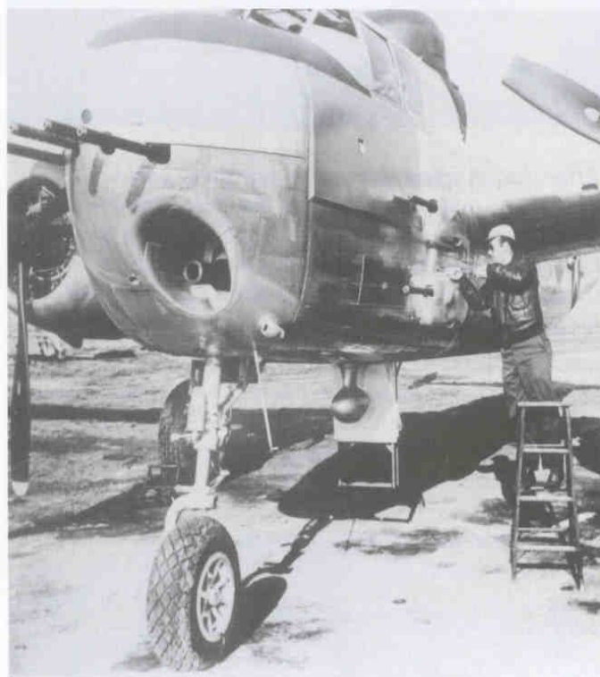
B-25H-1-NAs only had gun packs on the right side of the forward fuselage, but they were added to left side starting with the first B-25H-5-NA. Note the small round opening for the flush-mounted combat camera just above the four machine guns in the nose. The metal plate in the lower corner of the windshield on the pilot's side is also visible. (USAFM)
