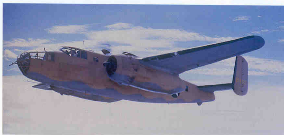
Left: By the time B-25Bs were in widespread use, the unit and aircraft numbers on the vertical tail had been replaced with the serial number which was stencilled in yellow. Standard practice was to delete the first digit of the serial number which was 4 for all versions of the B-25. (via Piet)
