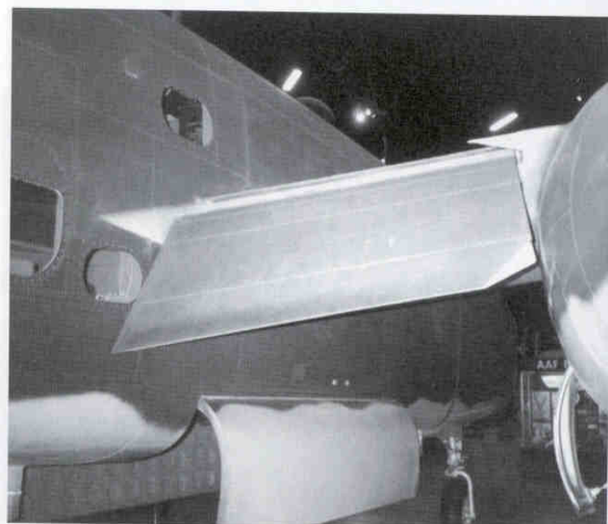
This is the right inner flap. This photograph, and the one to the left, provide a look at the scanning windows for the radio operator's position as found on the B-25D and F-10.
