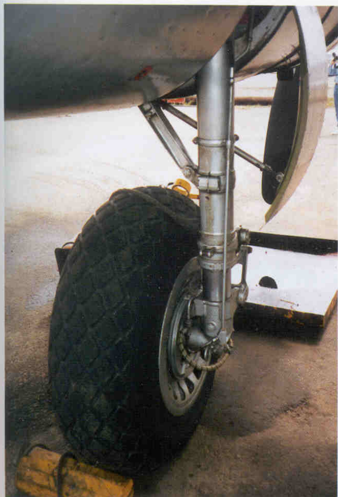
The angles between the strut, link, rod, and door are visible in this rear view. (IPMS Spruce Goose Chapter)
