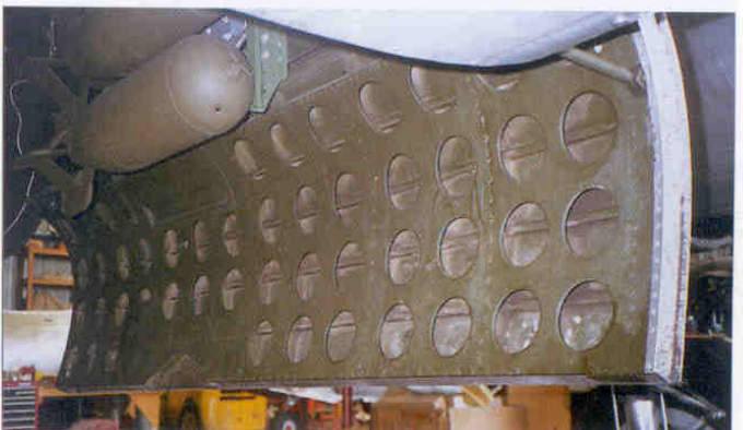
The left bomb bay door was simply a mirror image of the right door.
