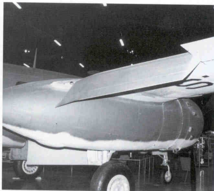
The outer right flap is shown here in the lowered position.
