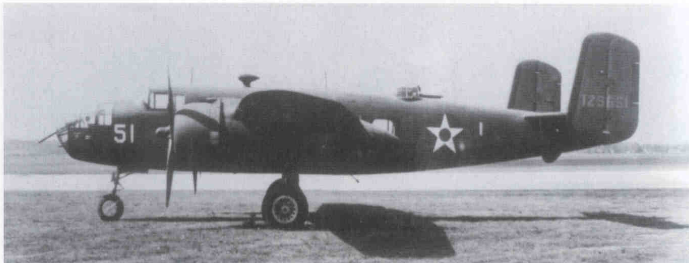
B-25D-NC, 41-29651, was the fourth D-model built, and it is shown here at Kansas City. It has been modified with large windows in the radio operator's compartment so that .50-caliber machine guns could be installed in the waist. Note that this early B-25D has the smooth cowlings as found on the B-25B. (National Archives)
