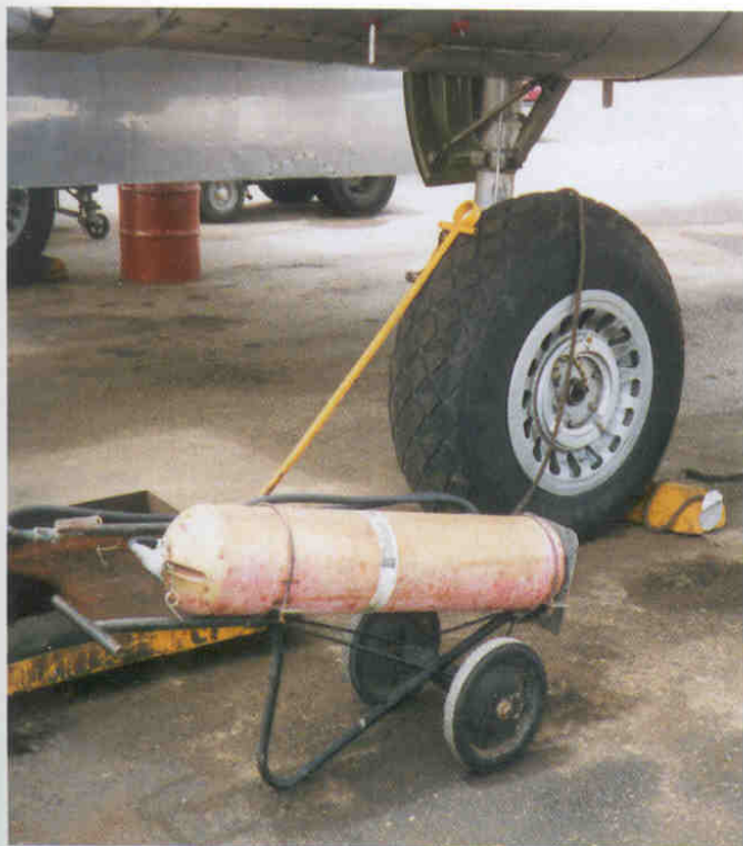
An overall photograph of the left main landing gear was taken during a maintenance period on the aircraft. This view clearly illustrates that only one small door remained open when the gear was fully extended. Again, open bomb bay doors can be seen in the background.
