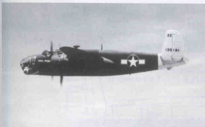
The F-10 was a photographic reconnaissance version of the B-25D. It had fairings for cameras in the nose, and additional cameras were carried in the aft fuselage. The gun turrets were removed. This F-10 was assigned to the 311th Photo Wing at Buckley Field, Colorado. After the war, F-10s remaining in service were redesignated RB-25Ds. (National Archives)
