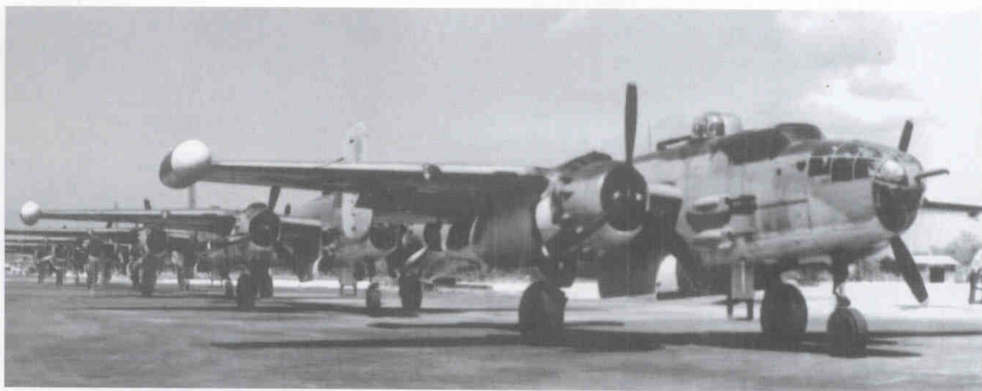
Above: These PBJ-1Js are painted in the tri-color camouflage scheme and have radomes on their starboard wing tips. They also have the bombardier's nose which was standard on most PBJ-1Js. (USAFM)
