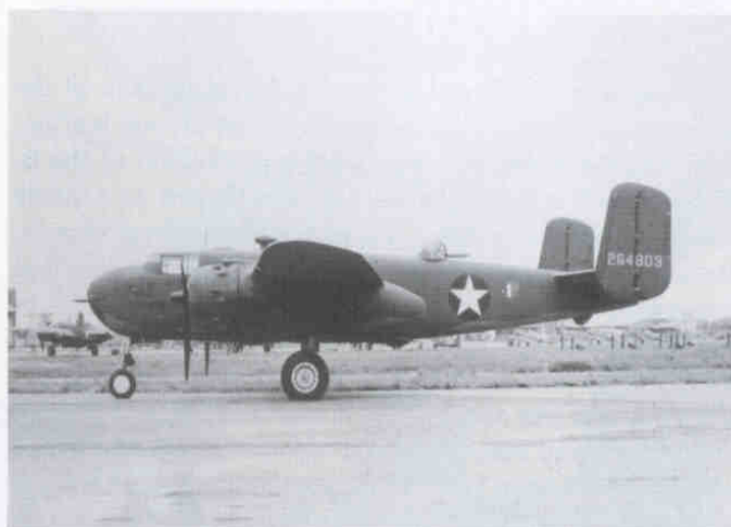
The B-25G and the B-25H had shorter solid noses in place of the standard bombardier's nose. A 75-mm cannon was mounted in the lower left side of the nose to augment the forward firepower of the machine guns. The B-25G, as shown here, also had two .50-caliber machine guns in its nose in addition to the 75-mm cannon. Strap-on gun packs on each side of the forward fuselage could add four more machine guns to the firepower. (USAFM)
