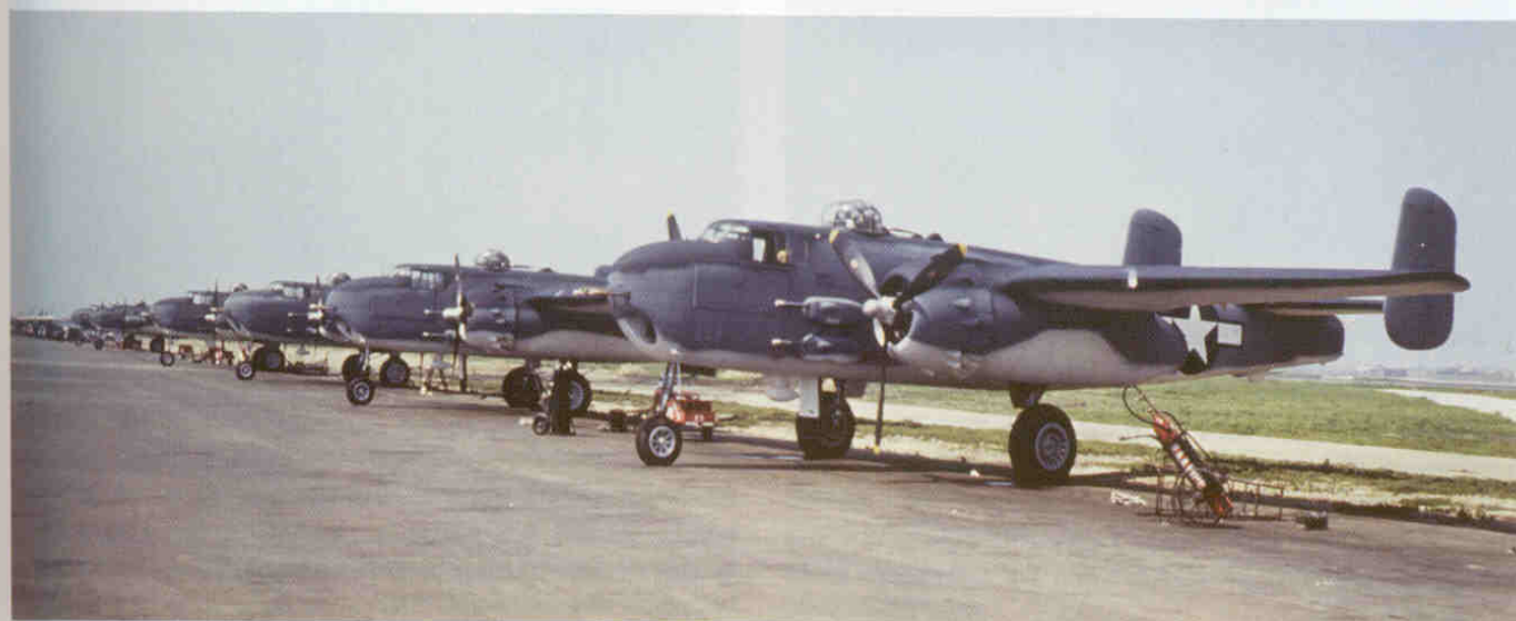
Below: This line-up of Marine PBJ-1Hs illustrates how the Navy applied its tri-color paint scheme of Dark Sea Blue, Intermediate Blue, and Flat White to many of its Mitchells. PBJ-1s seldom carried any unit or distinctive markings. (Varga collection via Piet)
