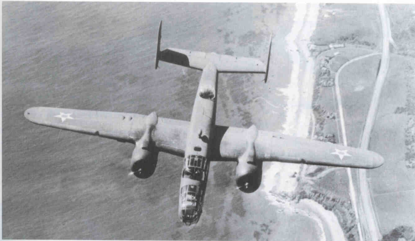
The top scanning window for the navigator's station, the ADF "football" antenna, and the manned turret are all visible on the top of this B-25B's fuselage. Also note the two small covers over the exhaust vents for the oil cooler ducts on top of the right wing. These were not present on the left wing. (National Archives)
