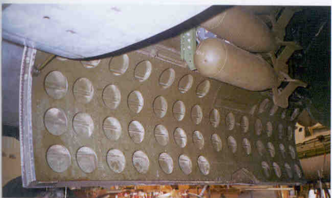
The inside of the bomb bay doors were perforated with numerous lightning holes.
