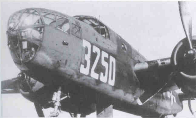
During the B-25C production run, the two side windows for the navigator's compartment were blistered slightly to improve visibility. The flat top window (not visible in this photograph) was replaced with an astrodome. (USAFM)
