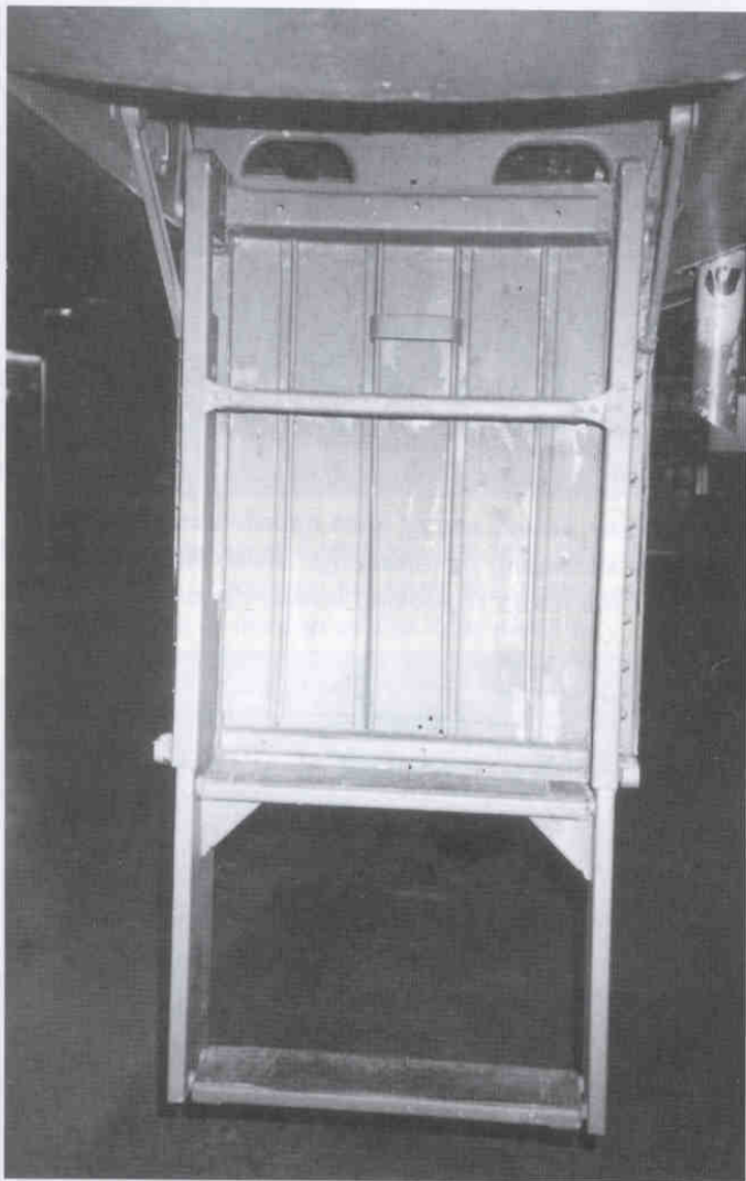
Entry to the Mitchell's forward and aft compartments was provided by two rectangular hatches under the fuselage that hinged at their forward end. Steps were built into the hatches to allow the crew members to climb up into the fuselage. This is the forward entry hatch as seen from the rear.
