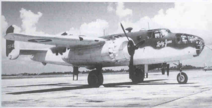
"Lady Jane" was B-25D-15-NC, 41-30409, and it was painted in an Olive Drab and white paint scheme used on sea search aircraft. It also has the astro dome and the bulged side scanning windows for the navigator's compartment. Note the later cowlings with the fairings for the exhaust stubs. Three recognition lights first appeared under the right wing tip on Mitchells during the B-25C and B-25D production runs. (National Archives)
