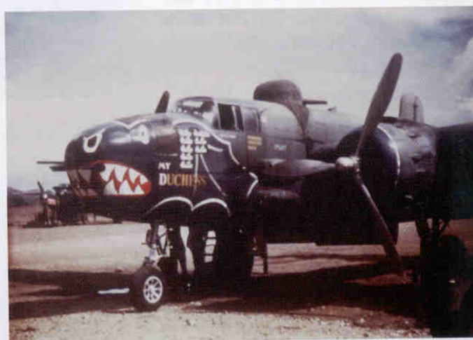
Some B-25Js assigned to the 499th BS of the 345th BG had elaborate art painted over the glass portion of their standard bombardier noses. "MY DUCHESS" was one such example. Two additional machine guns were installed in the left side of the nose compartment in an arrangement that mirrored the standard two guns on the right.
