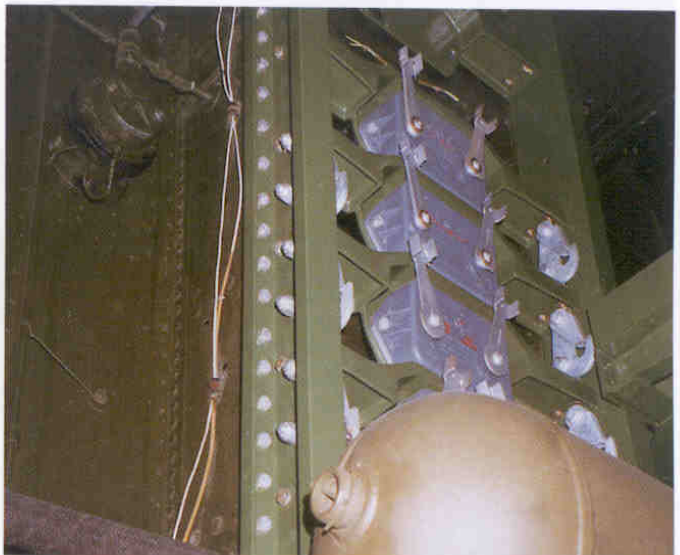
The bombs were attached to natural metal bomb racks fitted on the mounting structures. These racks varied in type according to the size of the bomb that was used. Three empty racks are shown here on the right side of the bomb bay.
