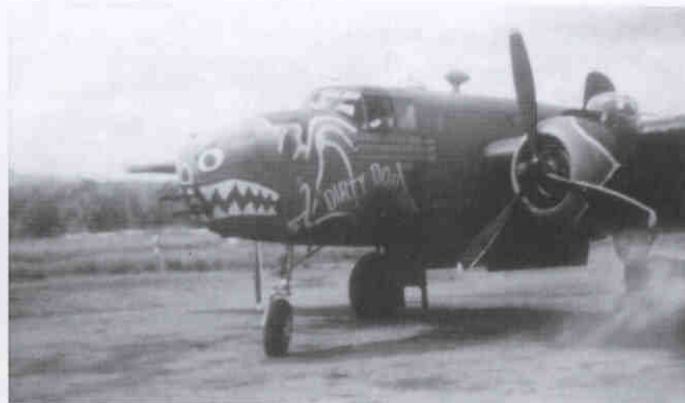
Some B-25Cs were modified to be used in the strafer role. The bomb sight was removed, and additional .50-caliber machine guns were added in the nose compartment. Although the standard bombardier's nose remained in place, it was often painted over with art as in this case on "DIRTY DORA." (Piet collection)
