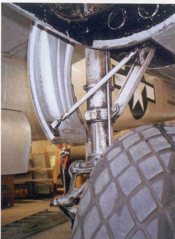
The connecting rod between the strut door and drag link is clearly illustrated here. Protective aluminum colored paint has been applied to all of the components of the gear except for the oleo portion of the main strut.
