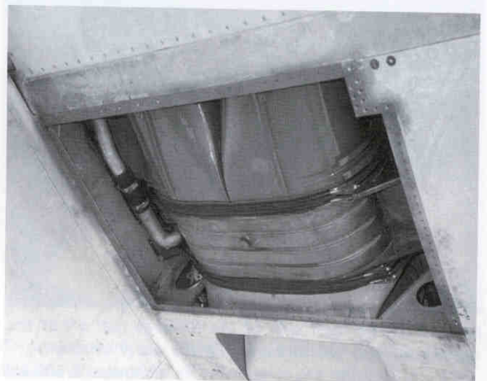
Above right: This is the left oil cooler, and again the access panel has been removed. A protective insert keeps foreign objects out of the scoop on the leading edge of the wing.
