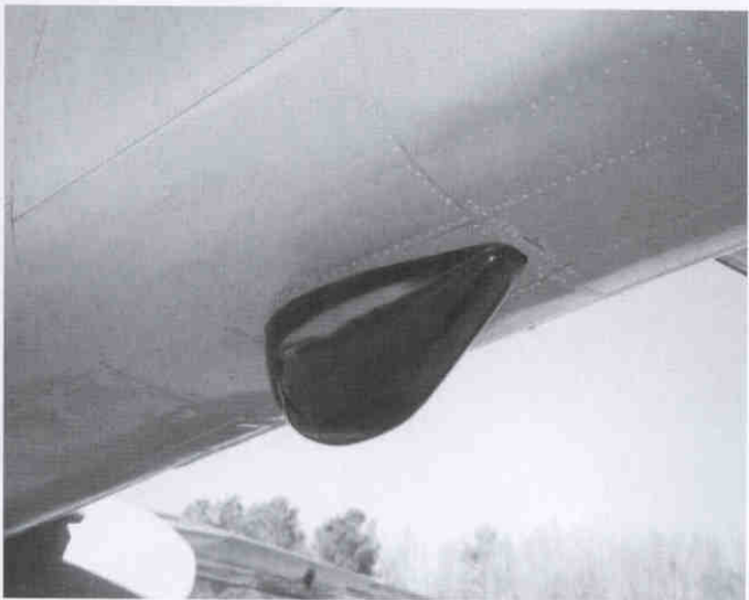
Beginning with the B-25C, a fixed tail bumper fairing became standard on all versions of the Mitchell.
