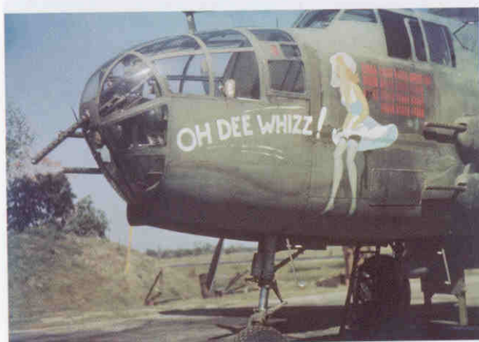
"OH DEE WHIZZ!" displays numerous mission markings indicating its service with the 63rd Bomb Squadron of the 12th Bomb Group. The nose of this aircraft is fitted with the single flexible .50-caliber machine gun and the two fixed guns on the right side. This arrangement was the production standard for B-25Js fitted with the usual glass bombardier nose.
