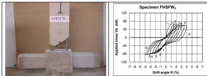
Figure 6: Plots of applied shear versus drift angle and failure mode of the strengthened subassembly FHSFW 3 .
