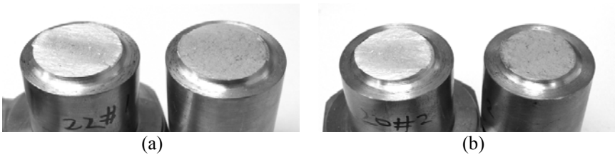
Figure 19: Typical fracture surface after dynamic shear tests: (a) D22; (b) D20.
