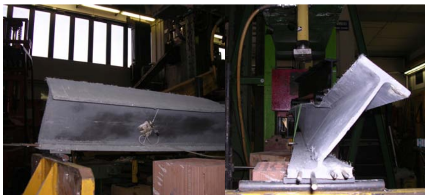
Figure 8: The RPC 200 beam after the bending test. No crack can be observed in the shear-stressed area (left) of the twisted section (right).
