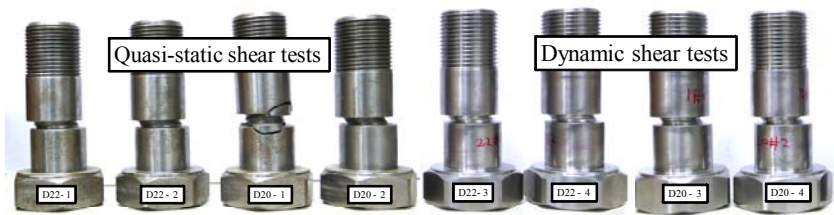
Figure 18: Deformed specimens after quasi-static and crash tests.
