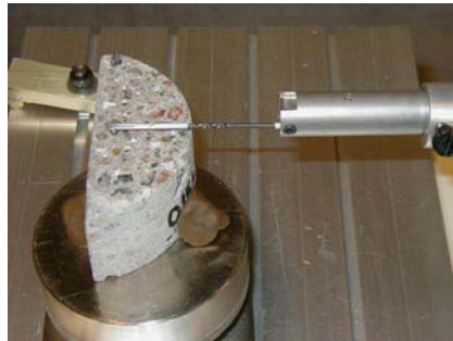
Figure 4: Stylus walking on the concrete surface.
