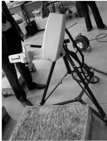
Figure 6: Testing system with camera CCD and parallel fringes pattern on surface.
