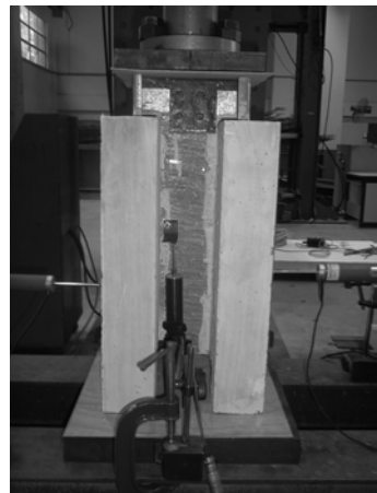
Figure 6: Push-out test arrangement.
