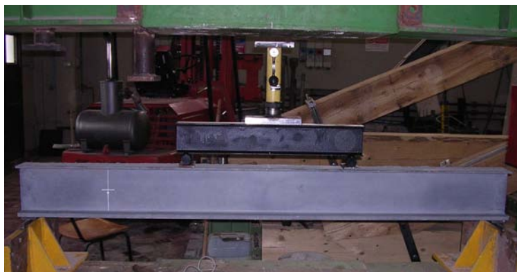
Figure 7: Four-points bending test on the RPC 200 beam.
