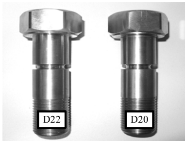
Figure 7: Prepared shear bolts.
